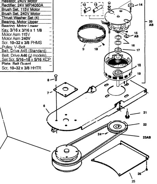
To tighten or remove the belt; Remove the belt guard, item 25, and loosen the (4) motor bolts, item 21. For additional information see page 4.
